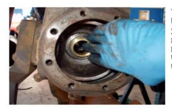
Toyota housings vary in size in the area behind the inner axle seal. Because if this, you will need to test fit the bronze insert that goes behind the inner seal. This bushing prevents the axle from moving around inside the knuckle and coming in contact with the trunion bearings.
