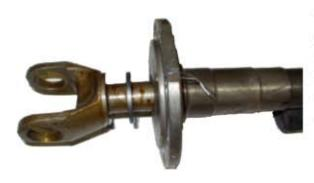
The thrust washer will ride against the back of the spindle and it keeps the axle assembly from moving side to side. Once the spindle is reinstalled and you have made sure the axle spins freely, you are done and can finish assembling the brakes.
