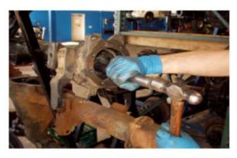
These bushings should be a moderate press fit. After the bushings are installed you can install the inner axle seals and the housing is done. Now that the housing is done you can install the universal joints and slide the axels into the housing.
