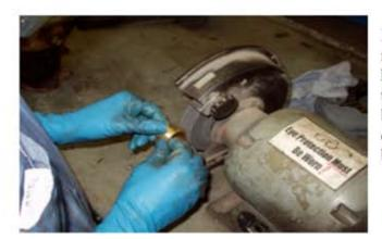
In most cases you will need to grind or machine the bronze bushings to fit your housing. Yukon gives you three bushings in this kit. You will only use two of these bushings, the third one is put in the kit just in case you make an error when grinding the bushings.
